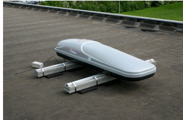
Figure 1: Typical HiSPARC detector
