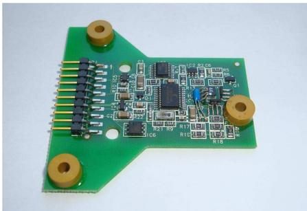
**Figure 4: B-field module with 3 Hall sensors**
