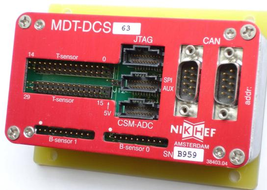
Figure 1: Picture of an MDM (112x60 mm)
