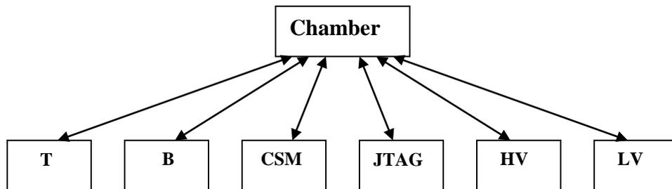
The chamber in this schema is the CU (control unit). It collects the status of the 6 sub-systems and derives a common status. A couple of remarks using this schema may seem appropriate:
